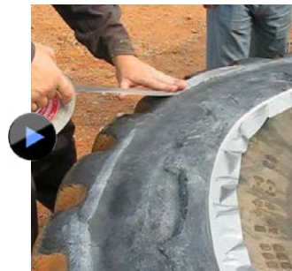
Video 7.2 Masking of edges with fabric tape
